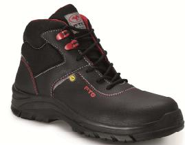
**Description** High shoe in black Safety-Leather with padded storm-cuff, 100% polyester lining, Non-Metallic HRP Insole , RELAX Insole, antistatic, breathable, mono density polyurethane sole , bending resistant , abrasion resistant , oil resistant , slip resistant , ESD.
